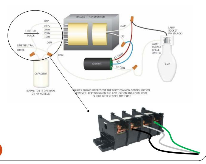
4. Remove Ballast, Capacitor and Starter from the fixture housing
