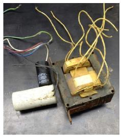
5. From the AC terminal block, wire the fixture to have a black or red wire (hot) run directly to the "pin" terminal on the Mogul Socket base. Wire a White wire (neutral) to run directly from the Neutral terminal on the block to the "thread" terminal on the Mogul Socket Base. Ensure the Fixture is grounded with the green wire.
